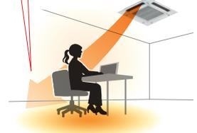
\*If people are present throughout the entire airflow range of an outlet, the airflow is shifted horizontally to avoid direct airflow.
