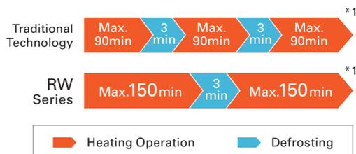
\*1 The time for heating and defrosting operation depends on the environmental conditions.
